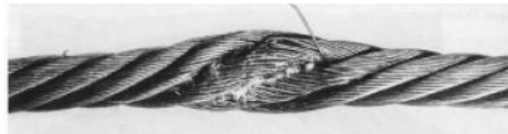
Wire rope with flattening caused by traversing
