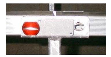
The patented Safe Fix pin system is a one step "insert and snap" method to assemble MODULO® platform components. The slotted pin is fixed in place by a spring mounted on the stirrup or U-frame.
